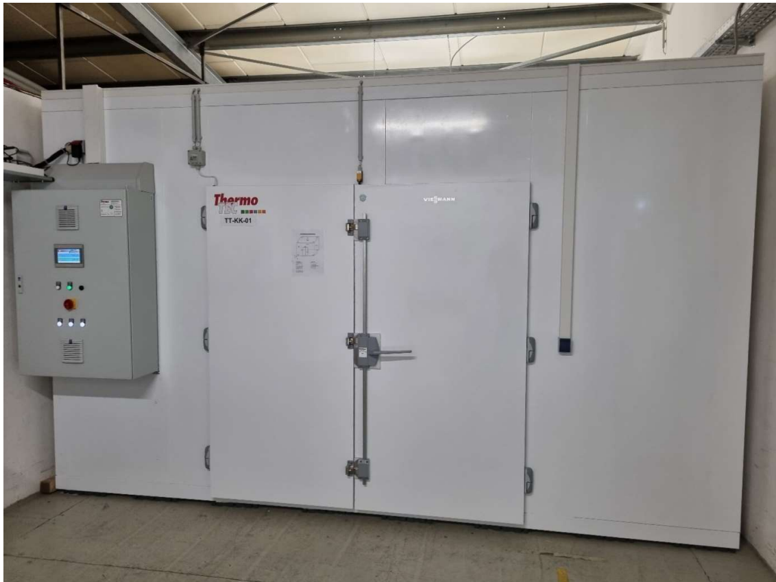
Front view of the new walk-in climate chamber. The available space was optimally and "tailor-made" utilized.
