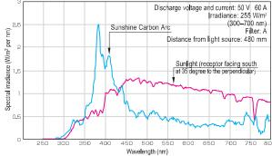
Trusted around the world for 60 years, this light source has an energy ascent in the ultraviolet portion very much similar to that of sunlight. Specified in many standards including JIS and ISO, its test results have contributed to the technological development of various products and materials. (P.9)
