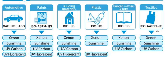
First and foremost, tests must be conducted with the right method for the specimen. The light source for each test is specified in their respective standards (page 15). It is crucially important for weather meters to perform a global standard test\* according to the international standard.
