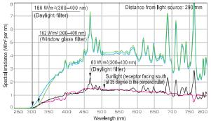
The spectral power distribution of this light source's irradiance in the ultraviolet and the visible portion is very much similar to that of sunlight. The spectral distribution of indoor and outdoor sunlight can be accurately simulated with the right combination of filters. The development of a new testing model capable of generating three times (180 W/m<sup>2</sup>) the irradiance of sunlight in the ultraviolet portion drastically improved the acceleration of its tests.(P.7,8)
