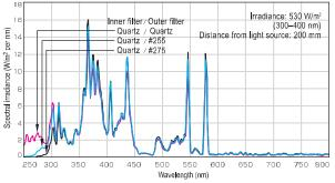
This light source produces ultraviolet energy that is much stronger than other light sources. It is developed for performing super-accelerated tests in order to meet the demand from today's high-speed product development. A research is in the process to determine its correlation with outdoor exposure.(P.10)
