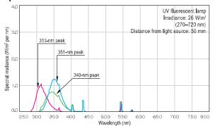
This ultraviolet fluorescent light source, with its peak in the ultraviolet portion between 280 and 315 nm (UV-B), is used in ultraviolet deterioration tests of paint and plastics. It is specified in ISO, ASTM and JIS standards.(P.9)
