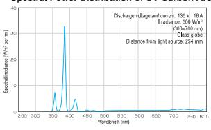
This light source, with strong energy in the ultraviolet portion (around 388 nm), is the oldest light source in history. It is widely used for lightfastness tests of everyday products such as textile products, interior appliances and stationery.(P.9)
